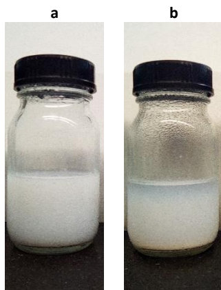
Figure 1. Photographs of a stable (a) and an unstable (b) nanofluid
