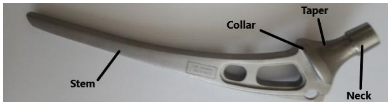
Figure 1. An example of a real hip implant with its components
