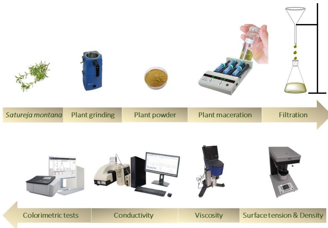
Figure 1. Flow diagram of the extraction process and the physico-chemical characterization of the extracts
