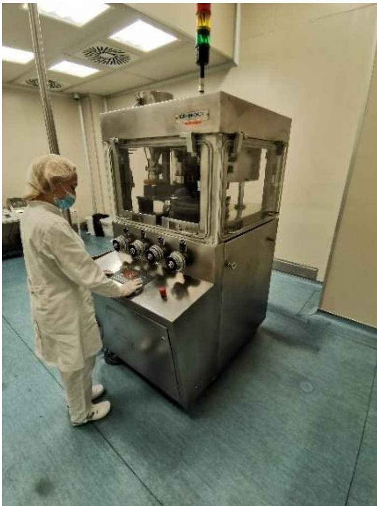
Mašina za tabletiranje (Horn Noack, Romaco Holding GmbH, Nemačka) Tableting machine (Horn Noack, Romaco Holding GmbH, Germany)
