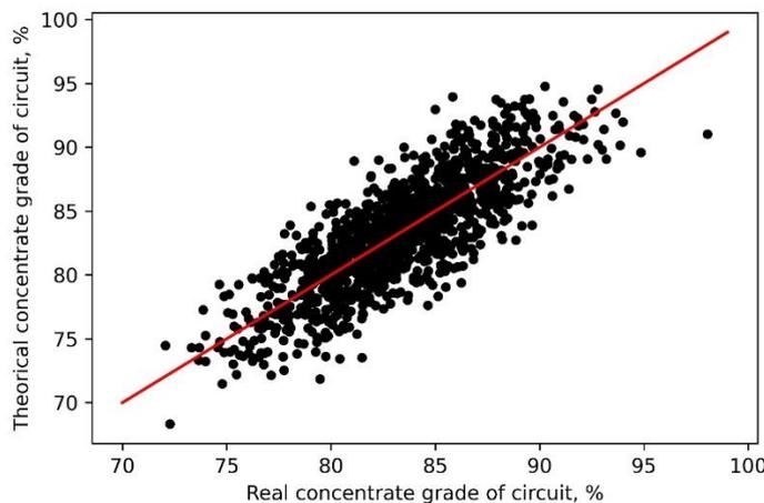
Figure 4. Real versus predicted mineral concentrate of the RCS circuit (output of the cleaner cell, Fig. 1)
