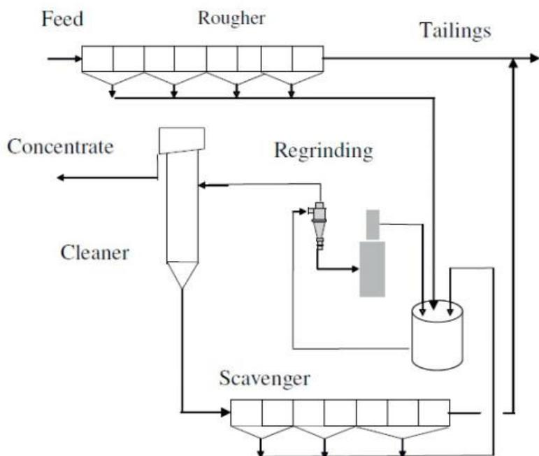
Figure 1. Structure of a high-level flotation circuit.
