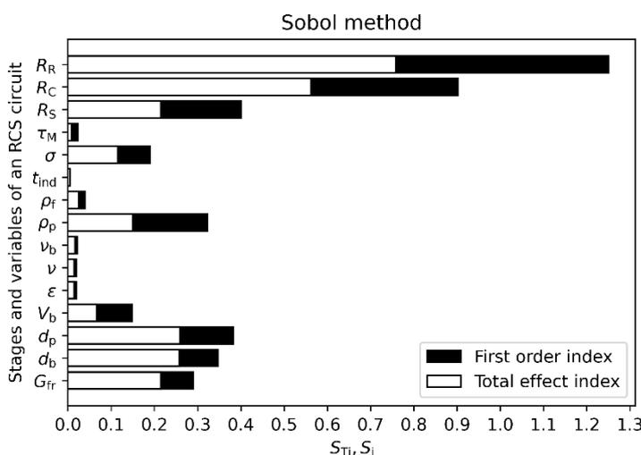
Figure 6. Average sensitivity indices calculated by the Sobol method in the RCS circuit.
