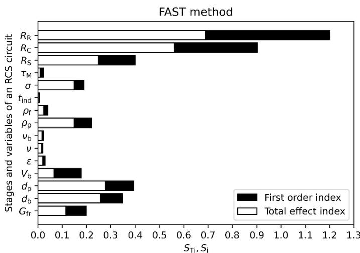
Figure 5. Average sensitivity indices calculated by the FAST method in the RCS circuit.
