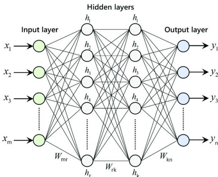
Figure 2. Multilayer perceptron architecture
