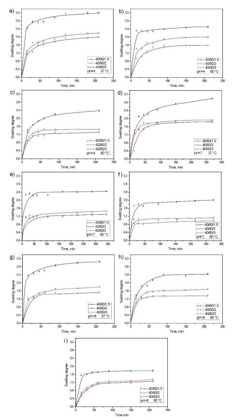
Figure 5. Dependence of the swelling degree of p(NIPMAM/NIPAM) hydrogels on time in the solutions at different pH values and temperatures: pH 4 (37 °C - a, 60 °C - b, 80 °C - c), pH 7 (37 °C - d, 60 °C - e, 80 °C - f) and pH 8 (37 °C - g, 60 °C - h, 80 °C - i); symbols connected with a smoothed line: experimental data (error bars are the standard error of the mean taken from three measurements)
