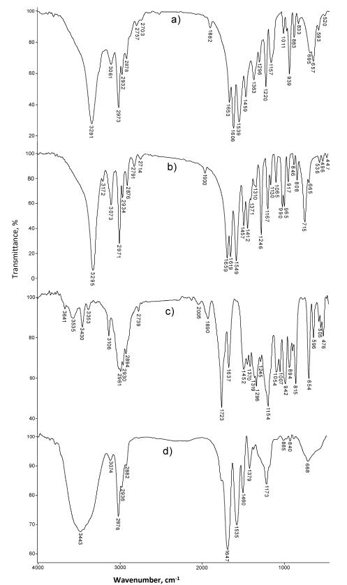
appears at 1459 cm<sup>-1</sup>. Consequence of C-H bond vibrations from the isopropyl group is an absorption band with the maximum at 1363 cm<sup>-1</sup>. The existence of the isopropyl group is indicated by the bands at 1157 and 1011 cm<sup>-1</sup>.
