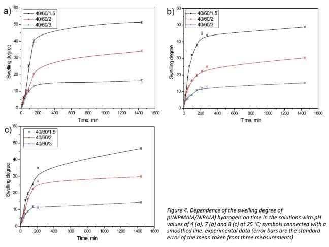
In mildly acidic environment (pH 4), hydrogels exhibited slightly higher swelling degrees as compared to the neutral or alkaline environment. Secondary amino groups of NIPMAM and NIPAM in the acidic environment can exist in the protonated state  $(NH_2^+)$ , which leads to the electrostatic repulsion of polymer chains and a higher degree of hydrogel
