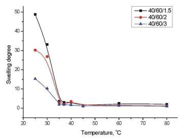
Figure 6. Dependence of the equilibrium swelling degree of p(NIPMAM/NIPAM) hydrogels on temperature in the solution of pH = 7
