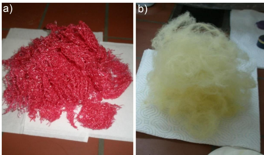
Figure 1. Photographs of tested polypropylene a - waste bag PPDJ; b - waste fibers from carpet production, PP
