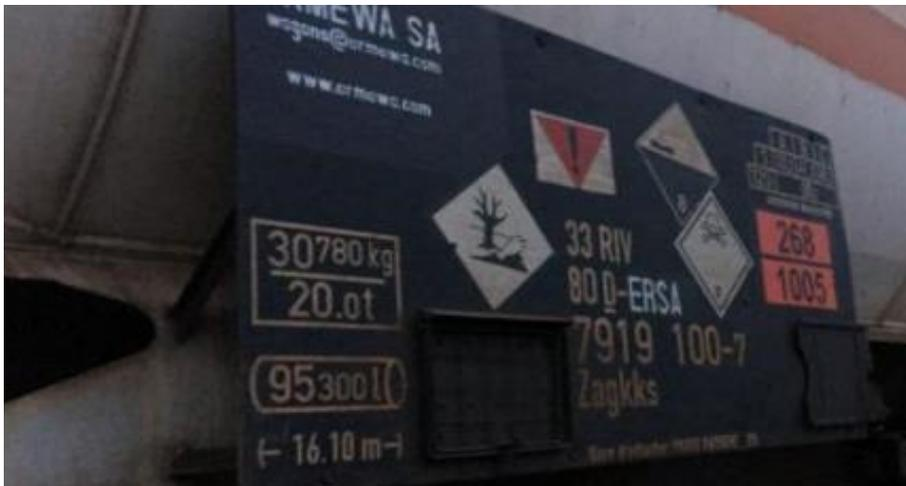
Figure 2. Specifications on tanks transporting ammonia
