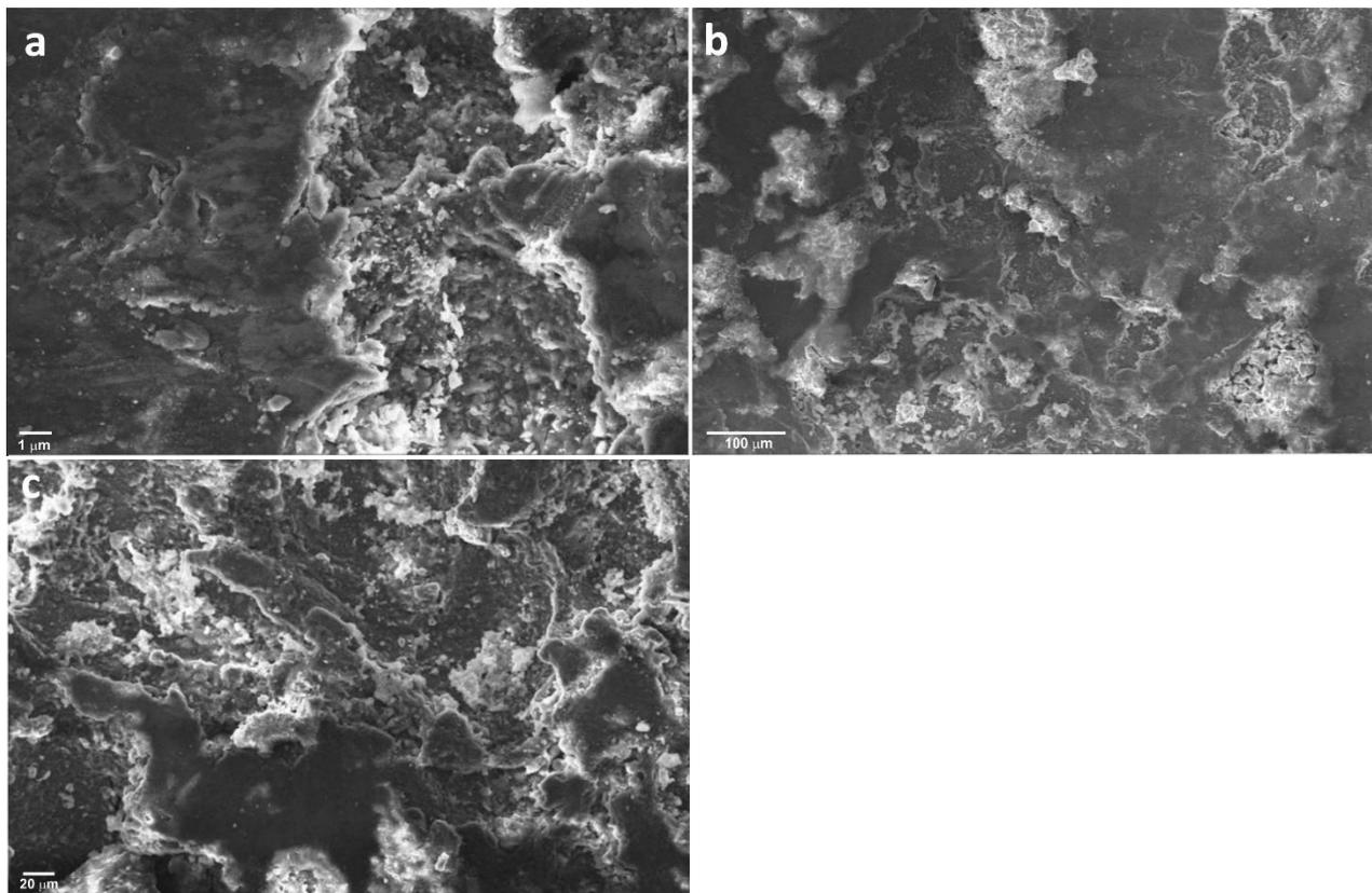
Figure 3. Microstructure of AZ61 Mg alloys reinforced with (a) 5 vol.% nano  $\text{Al}_2\text{O}_3$ , (b) 10 vol.% nano  $\text{Al}_2\text{O}_3$  and (c) 15 vol.% nano  $\text{Al}_2\text{O}_3$
