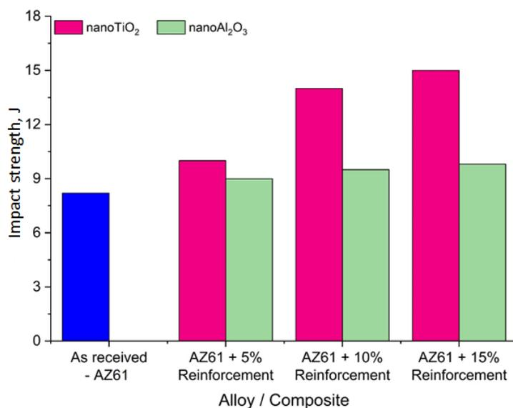
Figure 6. Impact strength of the non-modified AZ61 Mg alloy reinforced with nano- $Al_2O_3$  or nano- $TiO_2$  nanoparticles at different concentrations
