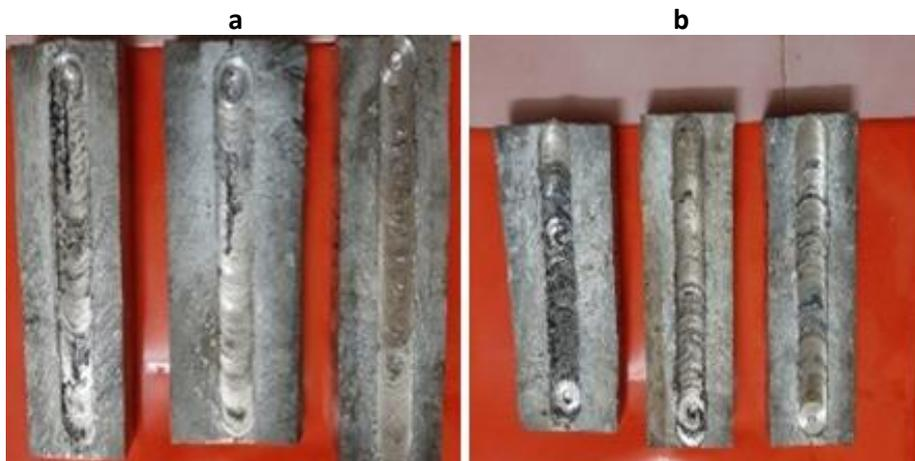
Figure 2. FSPed specimens with a) nano- $Al_2O_3$ , b) nano- $TiO_2$
