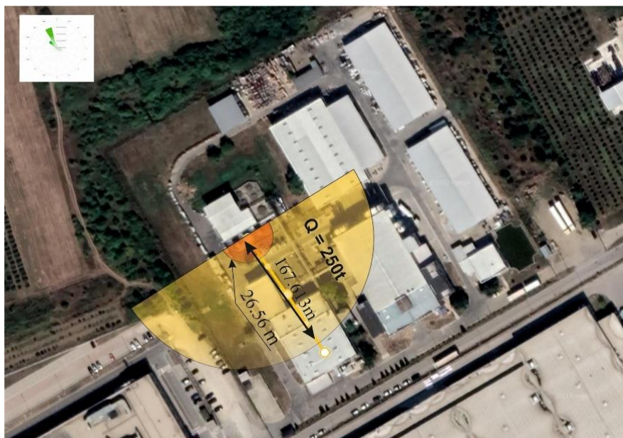
Figure 3. High lethality zone (orange) and irreversible effects zone (yellow) during the hypothetical leak of 250 t of carbon tetrachloride in a model paints and varnishes factory
