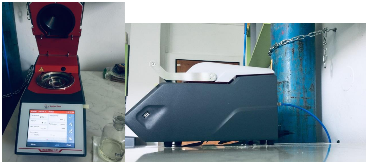
Figure D2. RapidOxy oxidation stability tester (RapidOxy 100, Anton Paar) at the University of Novi Sad, Faculty of Technology Novi Sad, Serbia
