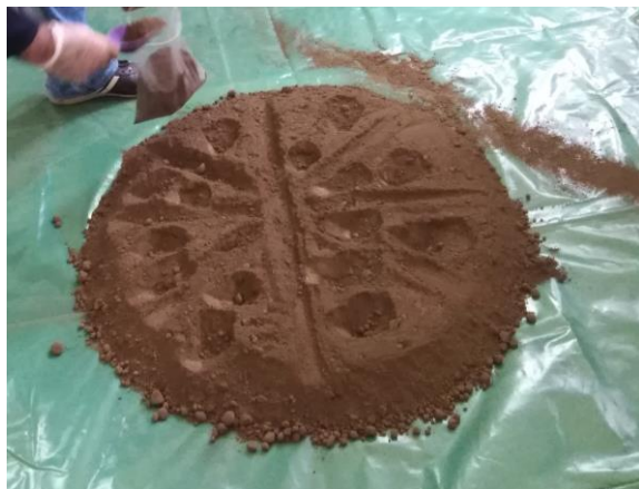
Figure 1. Preparation of the EAF dust representative sample
