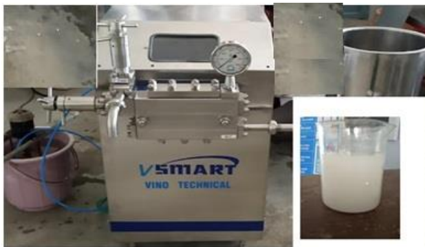
Figure 1. Preparation of \text{Al}_2\text{O}_3 -water-methanol nanofluid.
