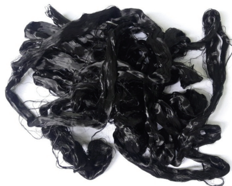
Figure 5. Photo of the filaments of the recycled polyester fibers with pigmentation of black masterbatches after 360 min of the beginning of the RTD test (wiring sample).
