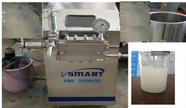
Figure 1. Preparation of Al 2 O 3 -water-methanol nanofluid.
