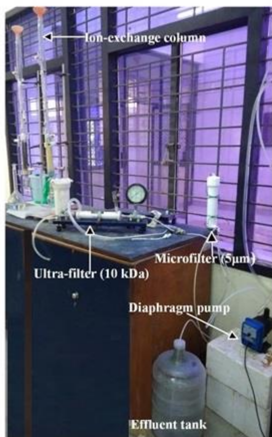
Figure 2. Bench-scale experimental setup.
