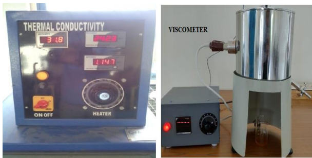
Figure 4. Measurement of thermal conductivity and viscosity of the \text{Fe}_2\text{O}_3\text{-W-EO} nanofluid.
