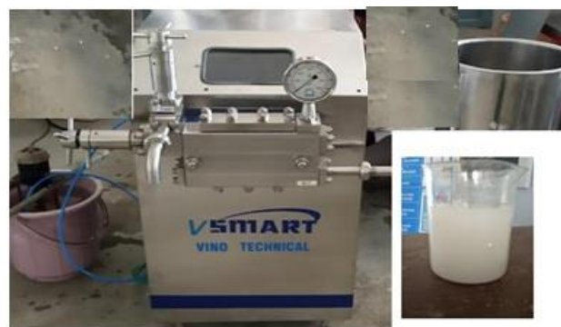
Figure 2. Preparation of the \text{Fe}_2\text{O}_3 -W-EO nanofluid.
